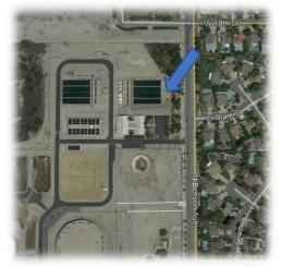
Justification: Install 16" pipeline connecting Company's existing surface water pipeline on Benson Avenue to WFA Facilities. The intent of this project is to allow San Antonio Creek surface water to be delivered straight to the WFA facilities. Delivering surface water to the WFA facilities will increase the Company's ability meet to entitlement for those stockholders that are members of, and receive water from, WFA; City of Upland, City of Pomona and Monte Vista Water District.
