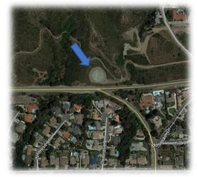
Justification: Reservoir 7 currently has a wooden roof that is in serious disrepair. Water quality issues require secure and safe roofing on reservoirs. The Company is planning on installing an aluminum roof to replace the wood roof. Installing a new roof will require installing a concrete perimeter, new access stairways and associated appurtenances.
