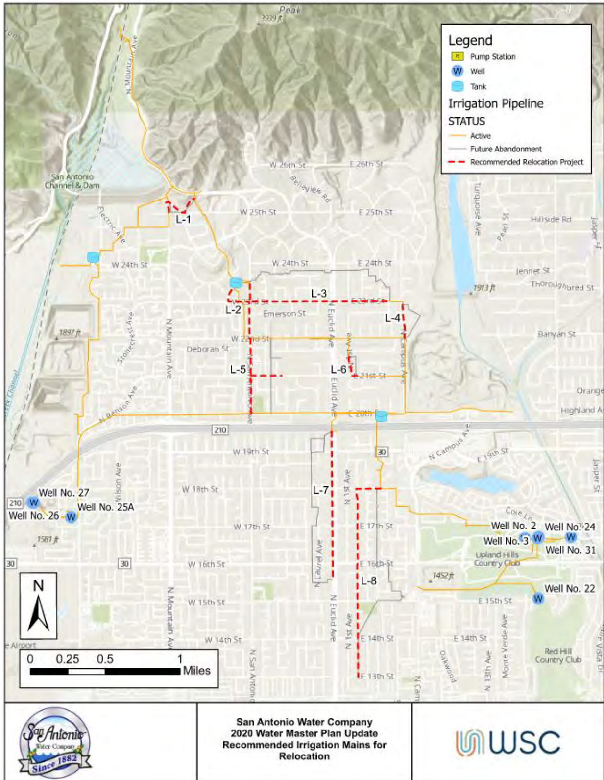
Figure 7-1. Recommended Irrigation Mains to be Relocated
