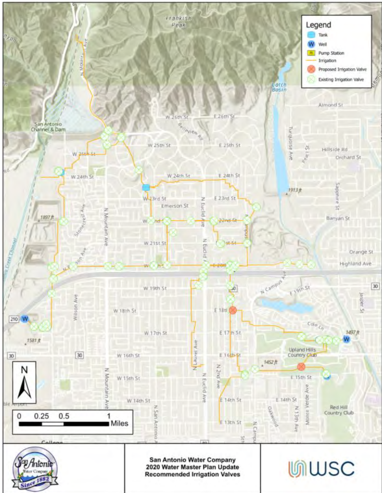
Figure 6-5. Recommended Irrigation Valves
