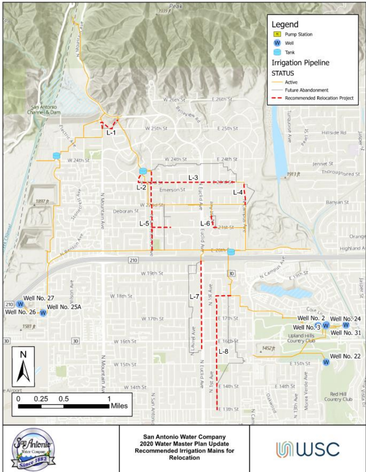
Figure 7-1. Recommended Irrigation Mains to be Relocated
