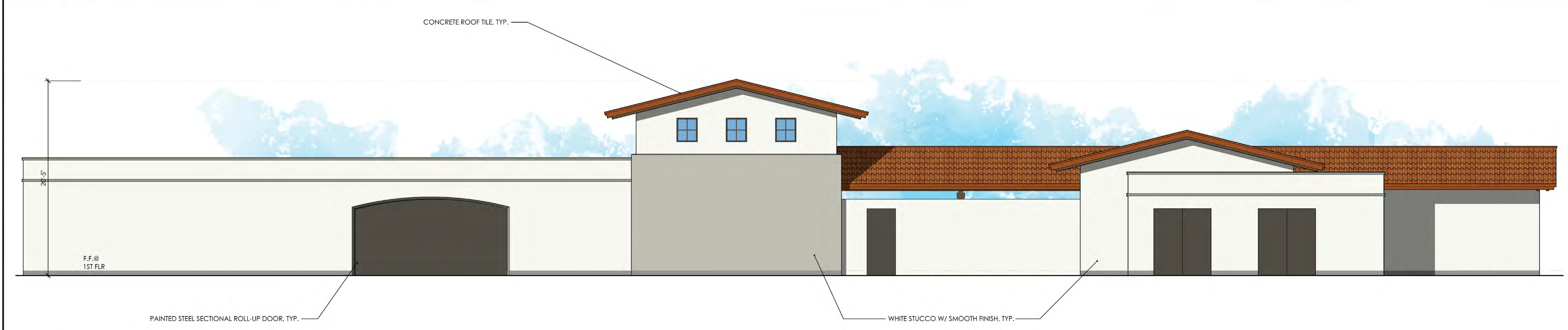
2 MAINTENANCE BUILDING SOUTH ELEVATION 3/16" = 1'-0"
