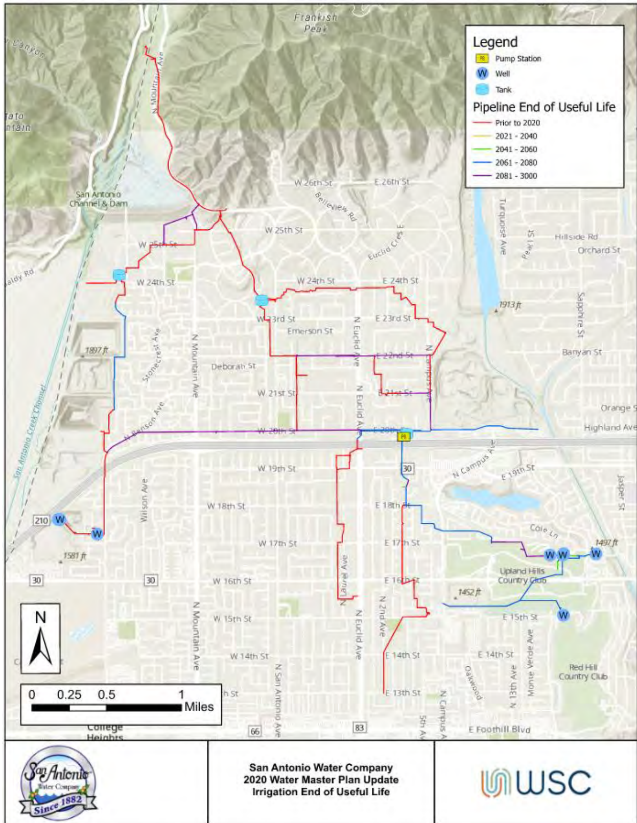
Figure 8-5. Irrigation Pipeline End of Useful Life
