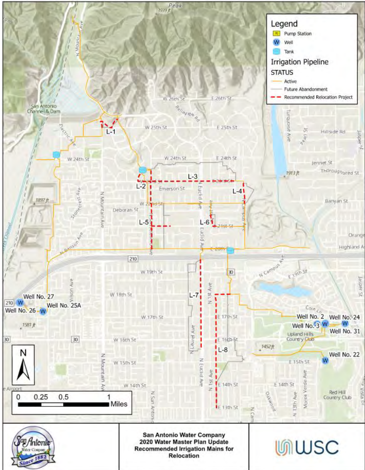
Figure 7-1. Recommended Irrigation Mains to be Relocated
