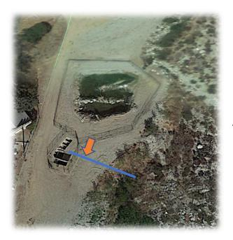
Justification: Current drain line drop gate is damaged and unable to hold back water. Water is passing under gate and discharging back to San Antonio Creek. Proposal is to purchase and install inline drain valve downstream of drop gate.
